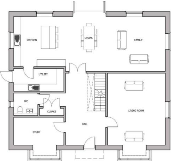
GROUND FLOOR PLAN
